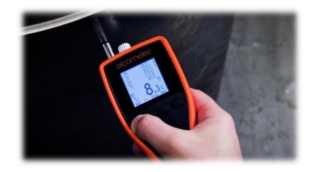
Purpose: The Elcometer 130 SSP is specifically designed to measure the level of soluble salts on surfaces, including abrasive media used in sandblasting. This device ensures that the abrasive material does not contribute to surface contamination that could affect coating adhesion.
