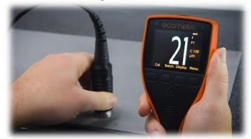
Purpose: This tool measures the surface profile (or roughness) after sandblasting. Ensuring the correct surface profile is essential for proper coating adhesion.
