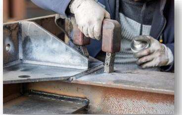
Ultrasonic Testing (UT): Use an ultrasonic probe to inspect the internal structure of the weld. This method can detect subsurface defects like porosity, lack of fusion, or inclusions.
