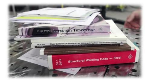
AWS D1.1 Structural Welding Code – Steel: This is one of the most widely used codes for creating WPS and PQR documents.
